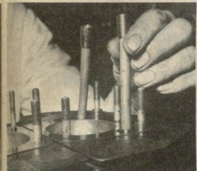
Two paper gaskets are used on the cylinder base joint. Put one on barrel and one on crankcase. The push-rods must be replaced with the shallow cupped end uppermost
