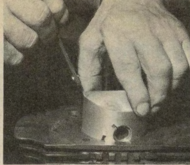
Clearance at the piston skirt must be .004 in. in all positions. The ring gaps should be checked and new rings should be inspected in the bore for flat spots (see text)
